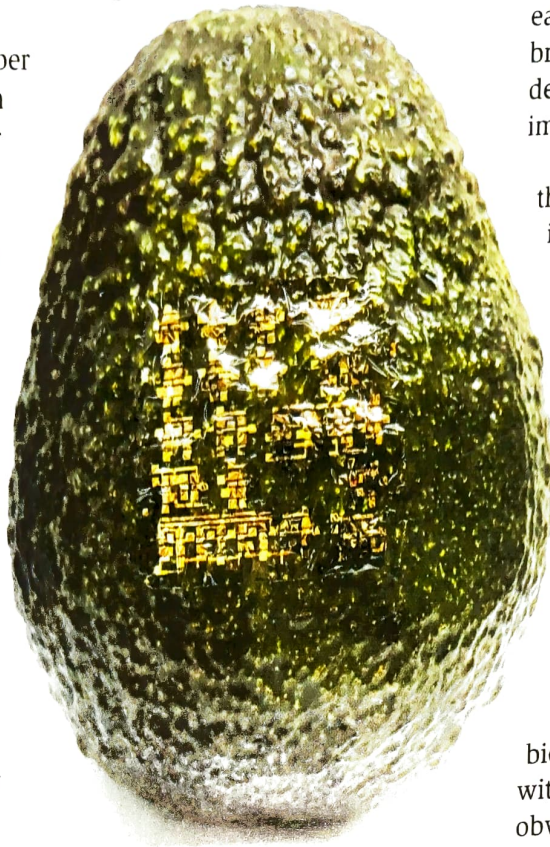
A new flexible and biodegradable semiconductor developed at Stanford University that can adhere to smooth or rough surfaces. Here it is shown clinging to an avocado! (Courtesy: Bao Lab)
